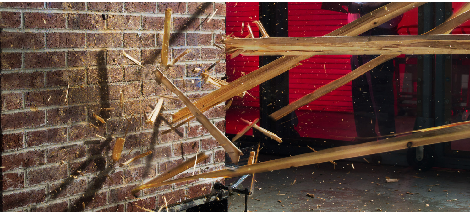
Tornado missile testing performed at Texas Tech University's National Wind Institute.
